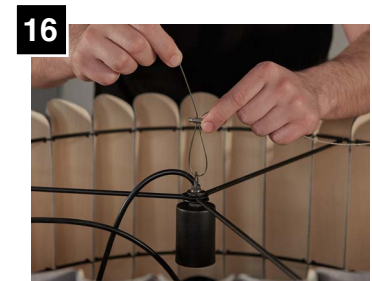
16 Continue to feed aircraft through remaining opening of strain relief.
